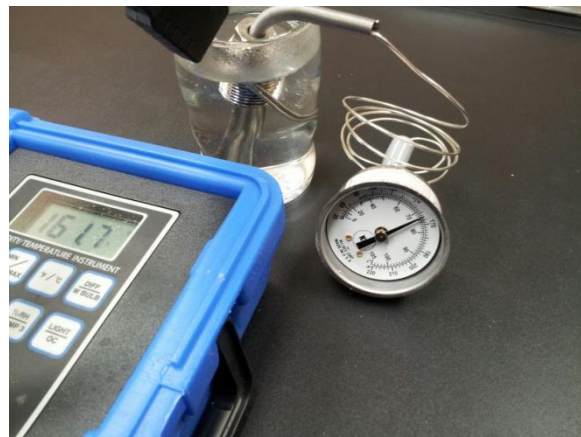
Test reading with known instrument, compare degrees
